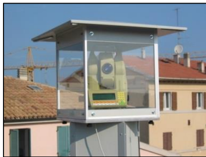
Topographic monitoring with high precision robot-supported station
